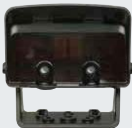
Radar movement detector MWD Fast and targeted automatic door opening, directional recognition, max fitting height 7 m, fitting in cold store possible up to max. 22°C, housing protection category IP 65
